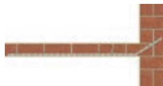
Reconnecting separated walls
